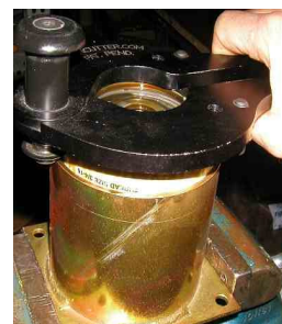
Figure 3: Cutting off the top
