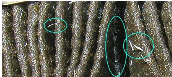
Small aluminum slivers from the piston pin plugs on a Lycoming O-320-H2AD engine.
