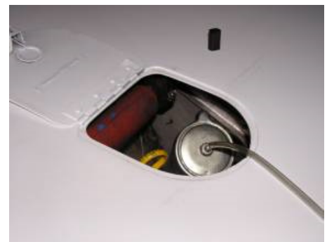
Air inlet fitting in oil filler cap.
