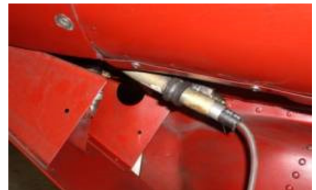
Pump return line installed in the blow-by port (in a Mooney 231).
