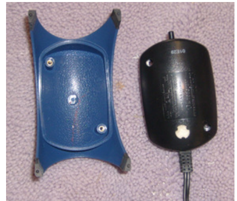
Disassembled air pump. Remove the felt filter in the bottom of the pump and plug the hole with glue.
