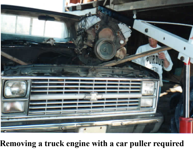
Removing a truck engine with a car puller required 2x4s, ingenuity, and nerve.
