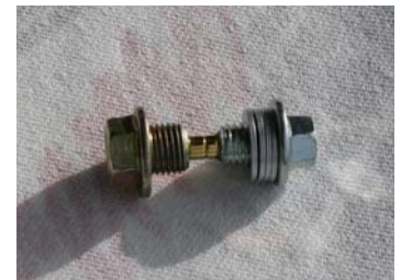
Figure 1: New magnetic drain plugs. Note the gold tip on each one.
