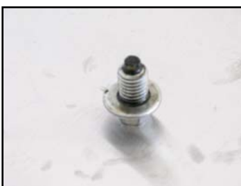
Figure 2: The Saturn's magnetic plug after one oil change. It's hard to tell, but the black is metal, not oil.
