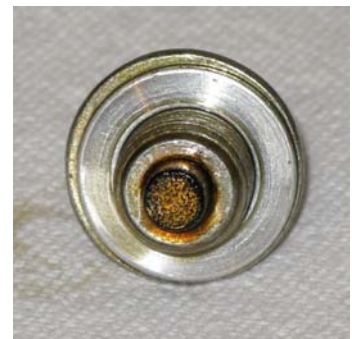
Figure 3: The Honda's magnetic plug after use.
