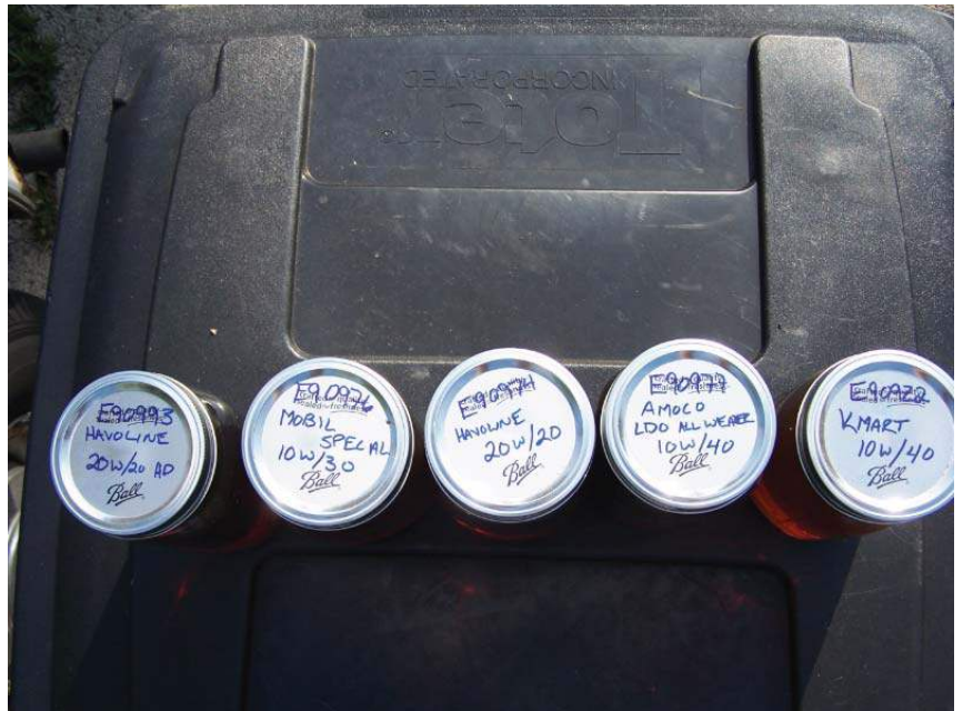
Figure 7: We are also not afraid of mixing oils. Next up: two quarts of Havoline 20W/20 and a quart each of Mobil Special 10W/30, Amoco 10W/40, and K-Mart 10W/40.
