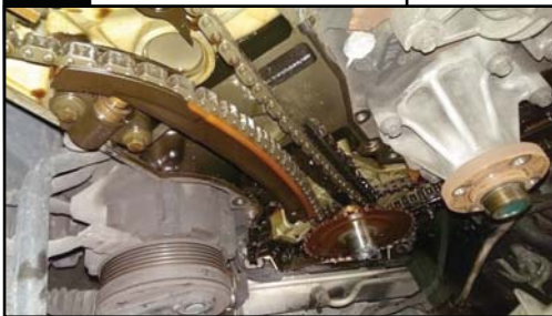
Broken timing chain tensioner
