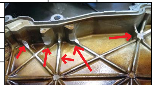
The worn timing-chain cover
