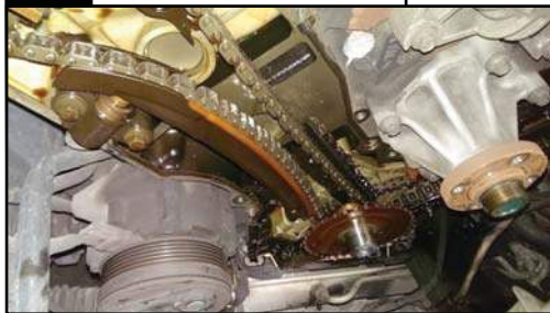
Broken timing chain tensioner
