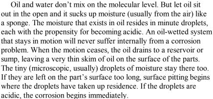
The additives in industrial oil tend to be alkaline in nature. They are usually sulfur or phosphorus compounds that will neutralize acids for long periods of use, as long as there isn't too much moisture present. After long-term use, traces of the additives can become free molecules that join with moisture to become sulfuric or phosphoric acids. It's bad practice to leave oil in place that will eat, rather than protect, the vital parts of a machine.
