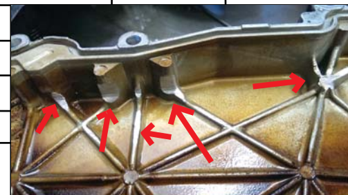
The worn timing chain cover
