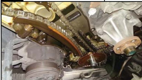
Broken timing chain tensioner
