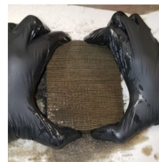
6. Squeeze pleats to remove oil if necessary.
