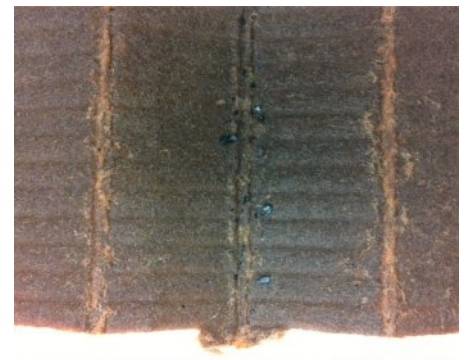
Carbon particles in filter pleat
