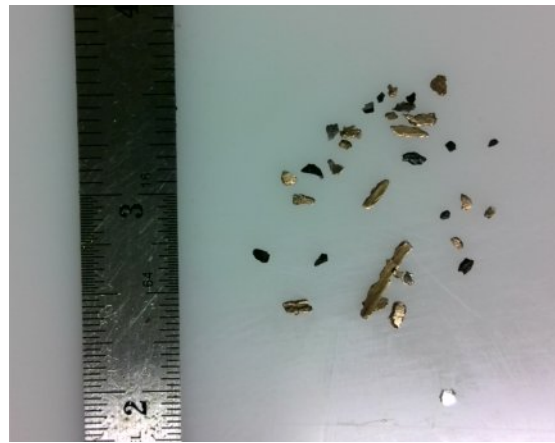
Mixture of brass/bronze particles and carbon
