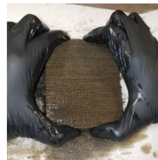
6. Squeeze pleats to remove oil if necessary.
