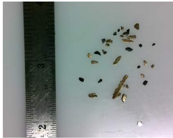
Mixture of brass/bronze particles and carbon
