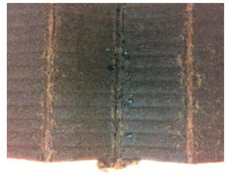
Carbon particles in filter pleat
