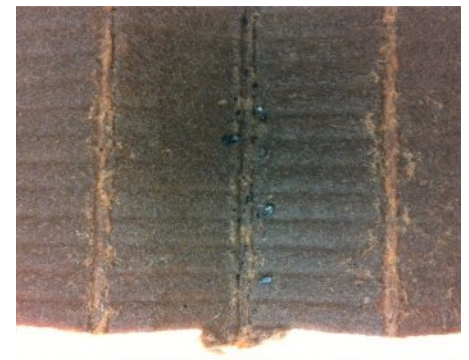
Carbon particles in filter pleat
