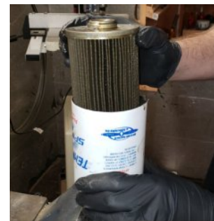
3. Cutting the filter lid and removing the pleats.
