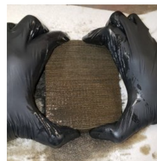
6. Squeeze pleats to remove oil if necessary.
