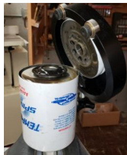
3. Cutting the filter lid and removing the pleats.
