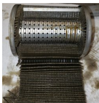
5. Cut pleats in the valley next to the filter seam (metal band) to remove.
