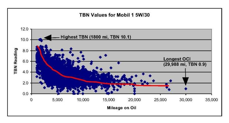
though we have many more TBN data points for Mobil 1 than we do Amsoil OE, the overall trends for TBNs are similar, and would be with just about any type of oil you could name.
