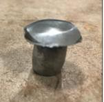
After receiving the 1/21 analysis with very high aluminum and finding a "loaded" oil filter, the owner had the engine inspected. He found excessive piston pin plug wear (see the picture above) as well as a worn front thrust bearing.
