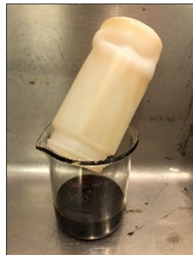
Image 1: Melted sample bottle. To our great surprise (and momentary panic) we learned our sample bottles melt at 392°F!
